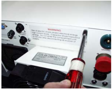
Removing Low Window Shield
