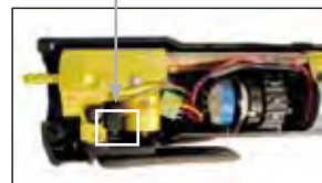
Trigger Sensitivity Adjustment Screw Location
