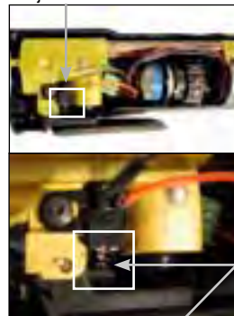
Screw adjusted out of trigger, pre-setting the micro-switch lever for shorter motion sensitivity.
